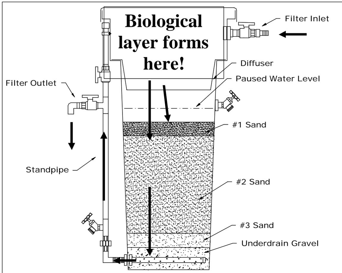
Figure 2. Cross-section of a typical low capacity demand operated slow sand filter.
